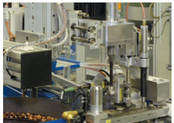
Automatic Installation of HELICOIL® plus M 8 SCREWLOCK®.
