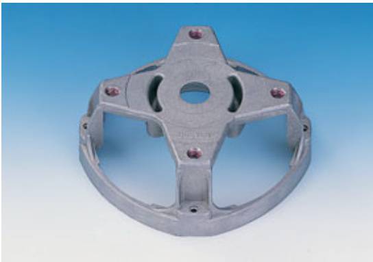
Engine support for garden chopper made from aluminium Screw loss safety device by means of HELICOIL® plus SCREWLOCK® M 8 x 12
