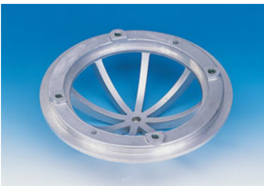
Drive over protection for a lighting fitting mounted into the ground. Material: aluminium die-cast HELICOIL® plus M 8 x 12 free running
