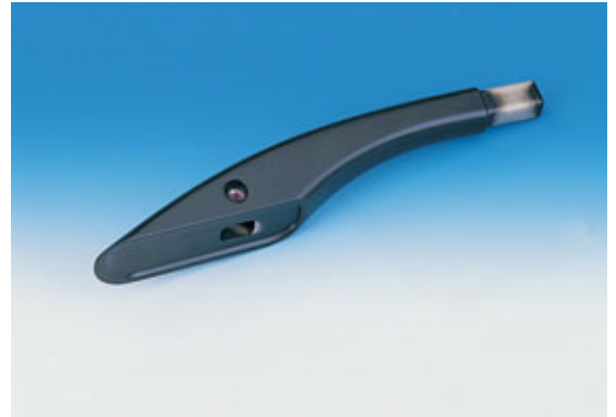
Car roof railing brace made from aluminium die-cast with HELICOIL® plus M 6 x 6 SCREWLOCK®
